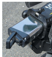
LEFT AND BELOW: The secret revealed: the battery pack is tucked away within the frame. It can be charged in place, or pulled out for charging away from the bike.
