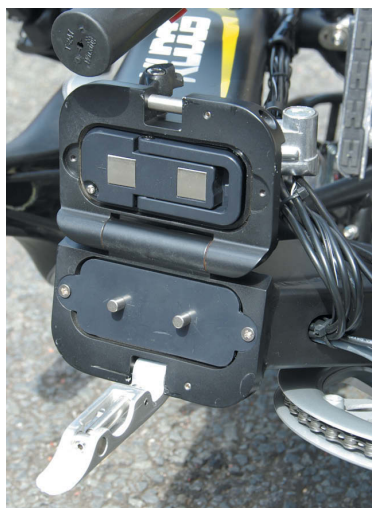
LEFT AND BELOW: The secret revealed: the battery pack is tucked away within the frame. It can be charged in place, or pulled out for charging away from the bike.
